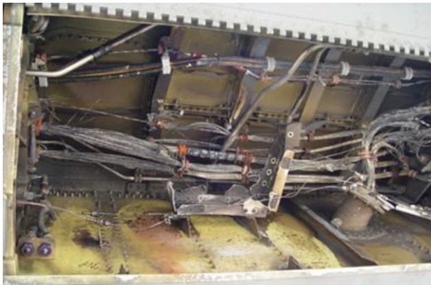
Fig. 6. In-flight electrical/hydraulic fire in an aircraft wing area [22].
